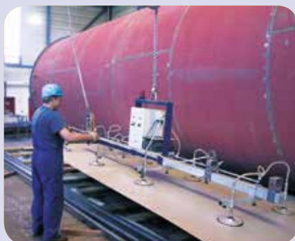
Mains-free lifter for sheet metal weighing up to 1,000 kg (AERO 1000/8R-24V)
