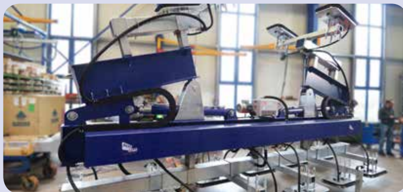
Stack-adaptable heavy duty device (hydraulically extendable)
