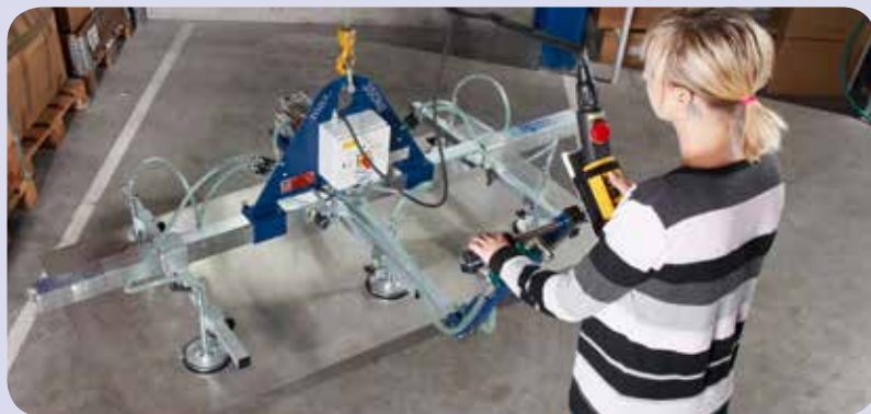
Good ergonomics due to adjustable grip design (grip down)
