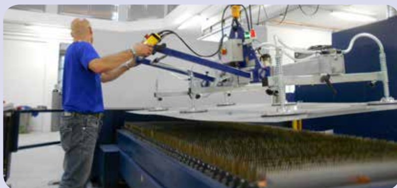
AERO 900/6R vacuum lifter for charging laser cutting systems
