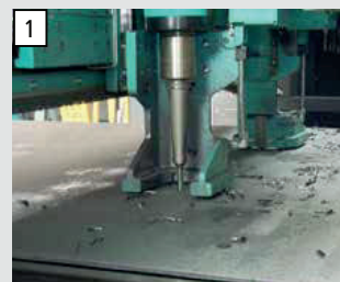
Second machining unit available as an option for increasing productivity by up to 100%.
