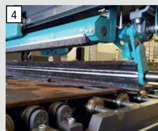
Prior to the thermal cutting process, a special brush removes swarf automatically and reliably to ensure good thermal cutting and reduce the risk of wear.
